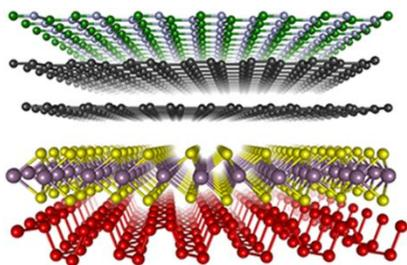
Scheme of a superstructure built from different two-dimensional crystals: going from bottom to top a layer of black phosphorus, of molybdenum disulphide, two layers of graphene and finally a layer of nitride of hexagonal boron are stacked.
