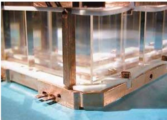
*Detail of the dioxide tellurium crystals of the experiment CUORE for the search of double beta decay without neutrinos.*
