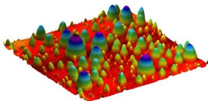
Atomic force microscopy image of a set of micro- and nano- hydrogen bubbles encapsulated by deformed layers of a MoTe<sub>2</sub> two-dimensional crystal. The side of the image measures 8 microns, and the maxim height is 100 nanometres.
