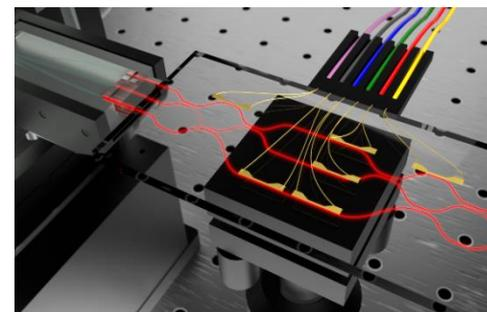
Schematic depiction of a quantum simulator made with integrated photonics. The single photons are sent inside the device and run through the several allowed paths made using waveguides. The operation carried out by the circuit can be programmed from the outside through electrical connections.
